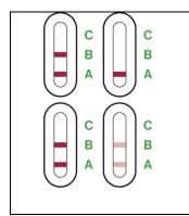
**Invalid:** No colored band appears in the control region (C), whether a test band(s) is present or not. Repeat invalid tests with a new sample, new test device and reagent. Insufficient sample volume, inaccurate operating procedure or expired tests may yield an invalid result. Contact your local distributor if the problem continues
