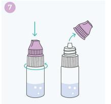
Tightly cap the buffer solution vial with the vial cap.
